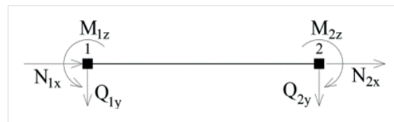
Fig. 3. Finite element (FE) under tension, compression and bending forces
